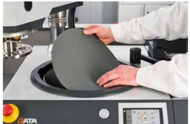
Placing e.g. grinding paper without adhesive/foil backing on GALAXY Quick-Tap
