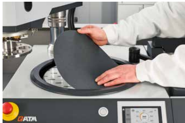
Placing e.g. a grinding paper with foil backing on the adhesive carrier disc
