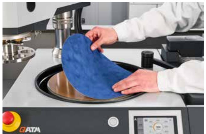
Placing e.g. self-adhesive polishing cloth on GALAXY X-Tap
