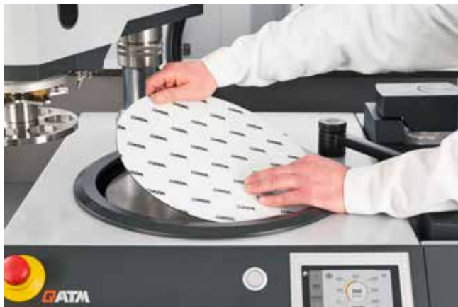
Applying the adhesive carrier disc
