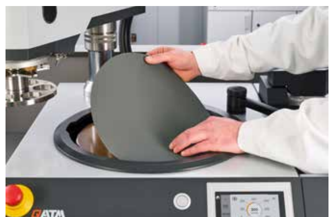
Placing e.g. self-adhesive grinding paper on GALAXY X-Tap
