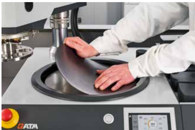
Applying the magnetic foil
