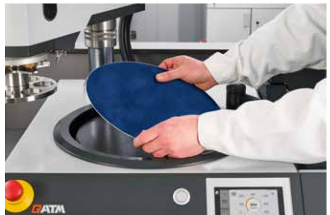
Placing e.g. a GALAXY polishing cloth on the magnetic foil
