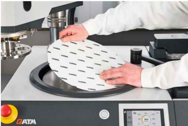
Applying the adhesive carrier disc
