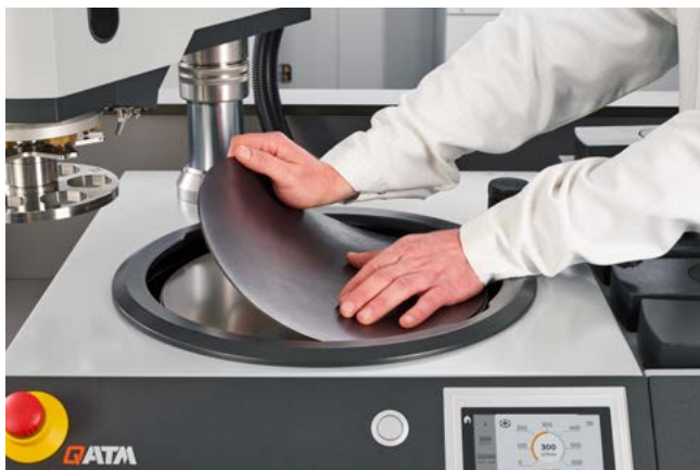
Applying the magnetic foil
