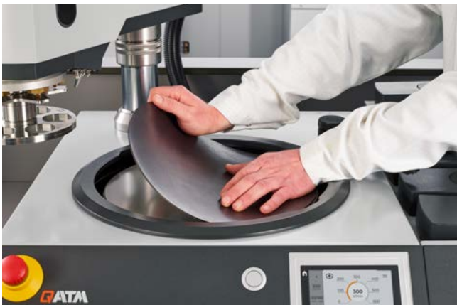
Applying the magnetic foil
