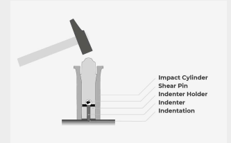
Integrated conversion for measuring the Brinell hardness of shear pin hardness tests, hammer blow method (shear pin - hardness testing) Suitable for steel and cast iron, conversion to HB 30, HRC, kg/mm 2
