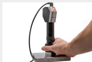
INDIRECT CALIBRATION USING A HARDNESS TEST BLOCK
