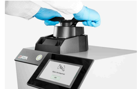
3. Lock the bayonet quick-release closure.
